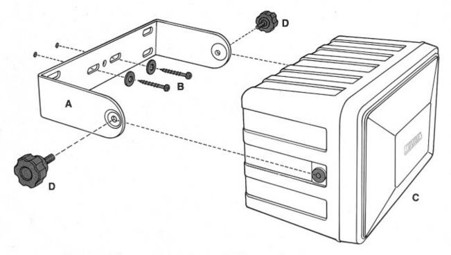
Installing the Bose® 121™ Mobile Monitor: The mounting bracket (A) is secured to the mounting surface by the recommended sized nuts, bolts and washers (B). The 121 Monitor (C) is then secured to the bracket by the supplied knurled knobs (D). Make sure that the lockwashers are in place on either side of the speaker, between the bracket and mounting holes.
