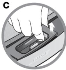
3. Press the dock release button (B) on the right and lift up (C) the right side of the dock to remove it.
