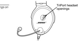
When wiping down the headset, be sure not to force any dirt or debris into the openings. Carefully use tweezers, if necessary, to remove foreign matter that may be lodged in the openings. Do not blow air into or vacuum the openings.
