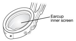
Do not attempt to remove, replace, or repair this screen. If operating problems indicate the need for screen replacement, contact the Bose<sup>®</sup> Aviation Headset Department. Refer to "Contact information" on page 34.
