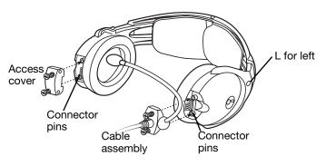
4. Press the assembly onto the connector pins until it is fully engaged and the cable assembly is flush with the earcup.
