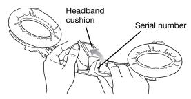
After locating your headset serial number, be sure to properly replace the headband cushion by pressing down firmly. For more information on replacing the headband cushion, see "Headband cushion replacement" on page 29.
