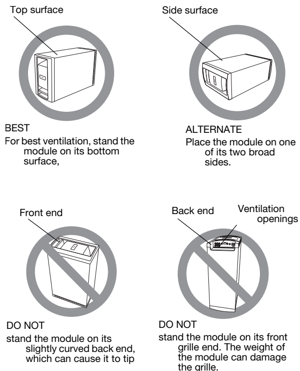
Figure 9 Proper and improper Acoustimass module positioning
