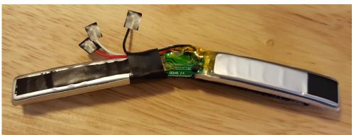
Dispose of the soft pack lithium-ion battery and the remainder of the product in accordance with local regulations.
