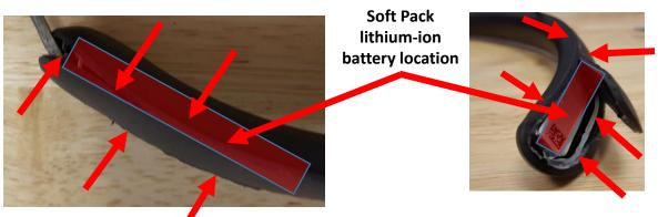
Note the soft pack lithium-ion battery location. Avoid damaging the battery while opening the product.
