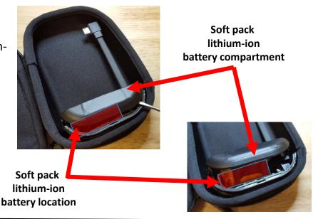
**(B)** Carefully remove the battery which is held in place by double-sided tape.
